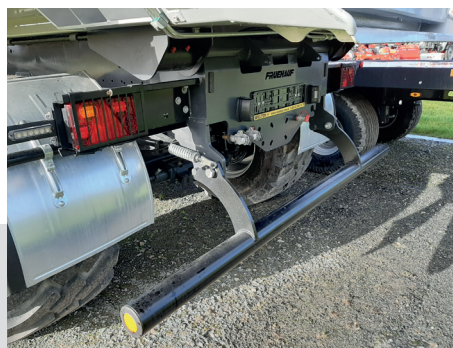
Barre anti-encastrément en position transport (modulable sans outil)
